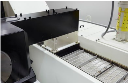
Automatic chip removal system
