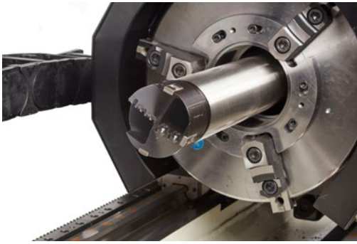
Standard heavy-duty 3-jaw chuck
