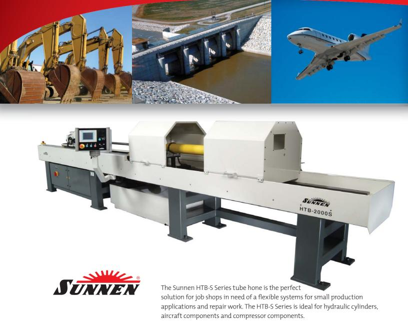
The HTB is available in seven models from the HTB-2000S [featuring a 2-meter (6.56 ft) stroke] up to the HTB-10000S [featuring a 10,000 meter (33 ft.) stroke]. These systems are designed for bore diameters up to 400 cm (13 in.)
